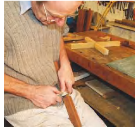
▲ Pic.14 Whittling a cylinder that fits tightly within the square void
